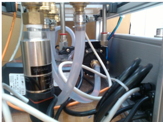
Figure 17 Hose for connecting the cooler
