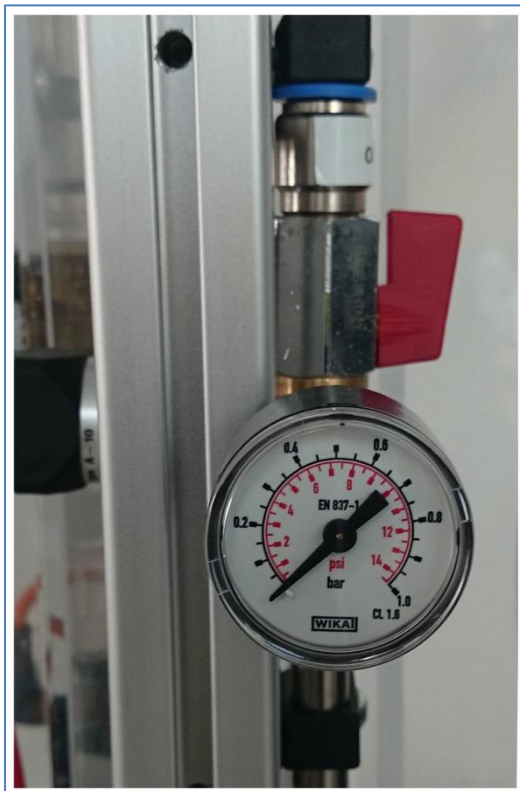
Figure 6 Optional pressure control behind the pump M3
